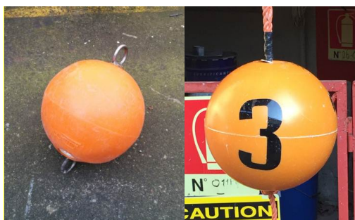
Figure 38. Image of the buoy without a number (gate) and with a number (plume). The OD of the sphere is 30 cm.
