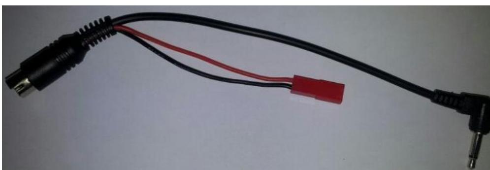
Figure 18. Buddy cable for EzUHF and Spektrum, JR, turnigy, Graupner, Fly Sky and Hitec radios.
