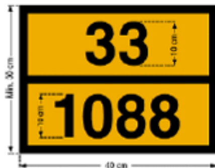
Figure 45. Example of an ERICard that will be positioned on the wall behind each valve.
