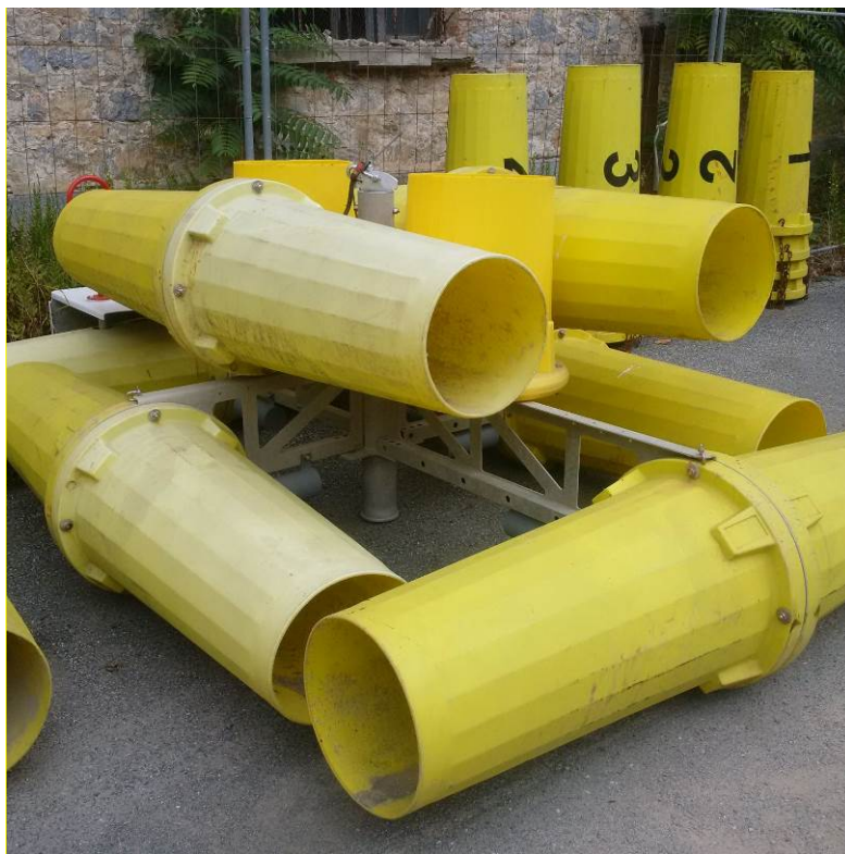
Figure 41. Piping assembly structure.. The structure, composed of yellow pipes, has the following dimensions: 2 m (front area) x 3 m x 1.8 m (height).
