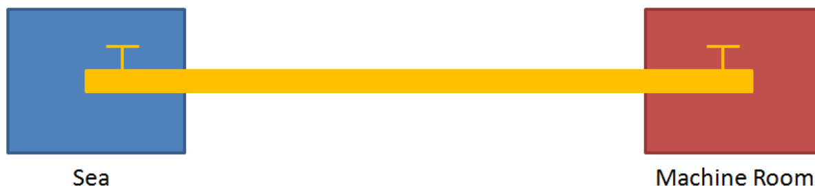
Figure 22. Each pipe has a valve in the machine room and another one underwater. (Source: ERL Emergency).
