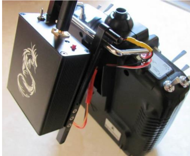
Figure 14. LRS module installed on a transmitter.
